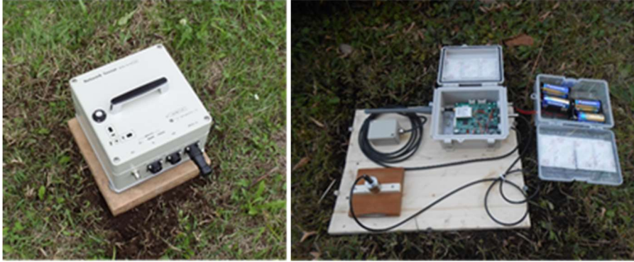
Fig. 2. (a) Conventional seismometer for comparison. (b) New type microseism accelerometer
